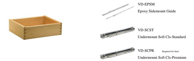
**Solid Maple Dovetail Drawers** sides and backs are 5/8" thick solid maple with a clear finish. The drawer bottoms are 1/4" plywood and are fully captured by the drawer sides, front and back. Dovetail joints are secured with adhesive and the bottom is secured with fasteners. Available guides shown below.
