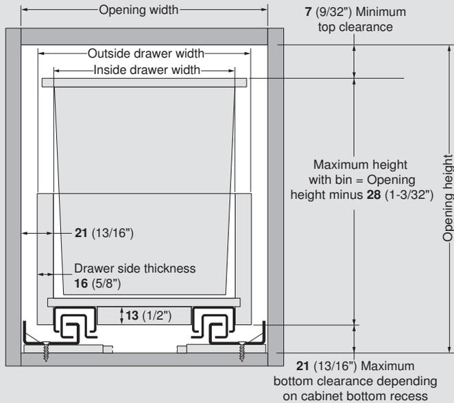
**NOTE:** Drawer side material thickness may vary. Accurate measurement of drawer side material thickness should be used when calculating outside drawer width using the table below. Inside drawer width **must** equal opening width minus **42 (1-21/32)** for MOVENTO runners to align and function optimally.
