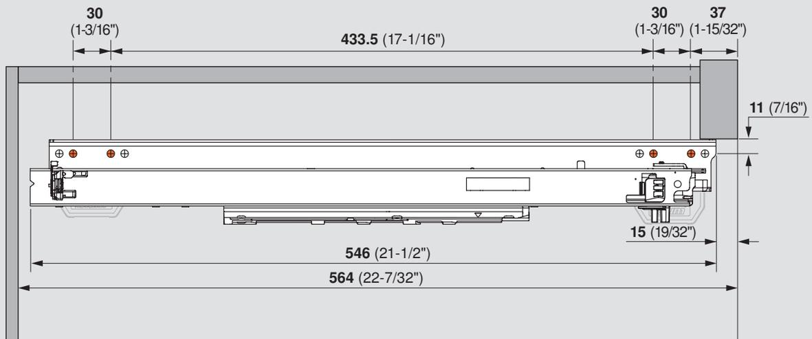
**NOTE:** Orange dots indicate pre-mounted screw locations. All four are required to meet specified load capacities.
